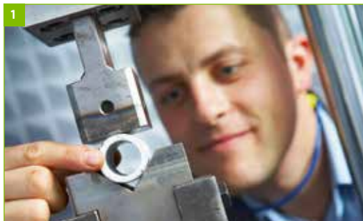
Illustration 2: Breaking load test up to 3000 kN
