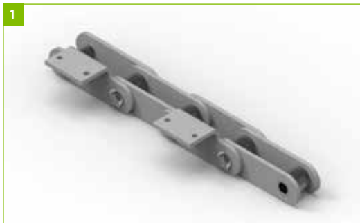
Illustration 2: Water ride chain with welded attachment angle and slide bearing in chain joint
