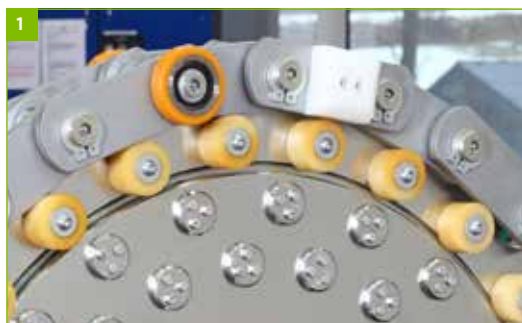
Illustration 1: Sprocket with noise dampening system
